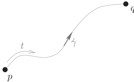
Figure 9.16 For a curve \gamma from p to q parametrised by the curve parameter t , we compute its length by integrating ds = \sqrt{g(\dot{\gamma}, \dot{\gamma})} dt along the curve.
