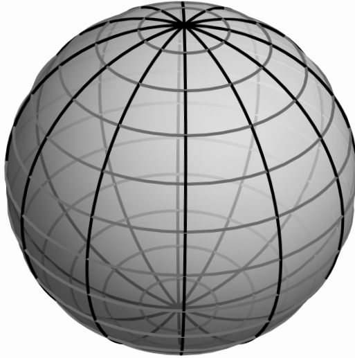
Figure 9.5 The \theta and \varphi coordinate lines on the sphere shown in black and red, respectively. The \theta coordinate lines correspond to keeping \varphi fixed and varying \theta and vice versa. The coordinate lines are also the flow lines of the coordinate basis vectors \partial_\theta and \partial_\varphi , respectively.
